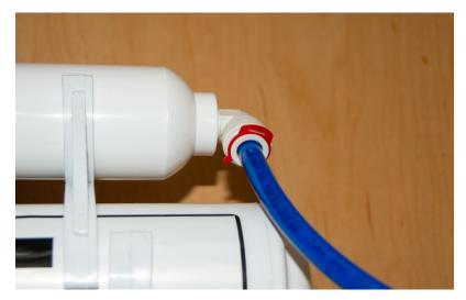
Locate the Red 3/8" tube and push into the post filter as shown below. Push the other end into the Ultrasonic Humidifier.
